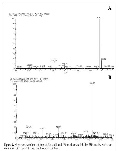
sampler, Finnigan photodiode array detector, and Finnigan LC pump (Thermo Electron San Jose, CA). Chromatographic separation was achieved with a Hypersil C<sub>18</sub> column (5 µm, 200- × 4.6-mm, Hanbon Science & Technology Co., Jiangsu, China). The mobile phase was methanol and 0.1% formic acid (80:20, v/v) with a total run time of 6 min. The flow rate was 1.0 mL/min, and the column temperature was 30°C.
