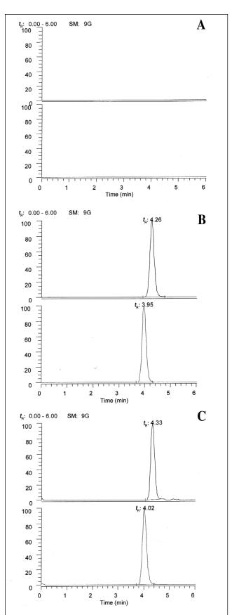
**Figure 4.** Typical chromatograms of paclitaxel in rat plasma: blank plasma (A), plasma with paclitaxel (50.2 ng/mL) and docetaxel (640 ng/mL) added (B), and plasma with docetaxel (640 ng/mL) added 15 min after being administered with a single dose of taxol and paxlitaxel (5 mg/kg) (C).
